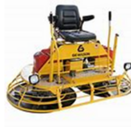
Ride on Trowel Machine for finishing much larger areas.
